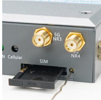
Step 2: Insert a SIM card into the SIM tray. Close the SIM tray, ensuring it is seated back in place.
