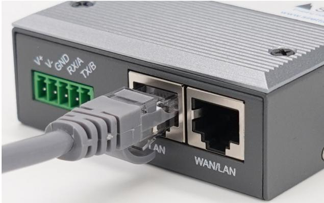
Step 5: POWER: Plug the green power connector on the power adapter cable into the router as shown below. Plug the 2.1mm centre pin connector from the plug-top power supply in to the other end of the power adapter cable.
