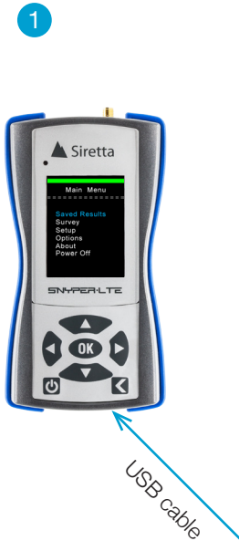
Figure 26. Connecting USB cable
