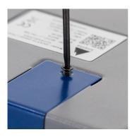
**Step 2:** SIM: Insert a SIM card fully into the SIM slot. Close the SIM cover, ensuring it is screwed back into place
